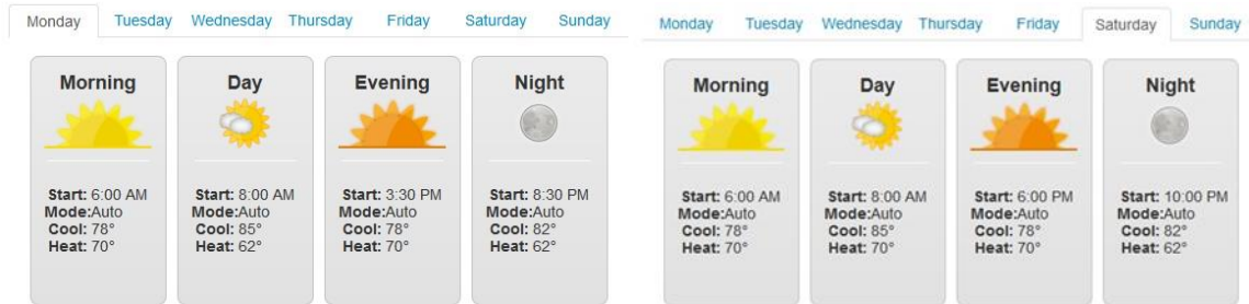
Figure F-4. Screenshots of programmed thermostat settings for Participant 2 (Thermostat 1), taken on January 8, 2013
